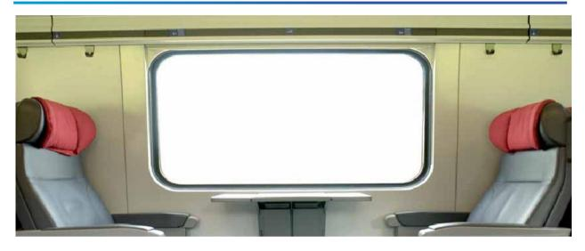
SABIC's ultra-tough, flame-retardant (FR) LEXAN<sup>TM</sup> F6000 polycarbonate (PC) sheet has been chosen by Plexx AS, a leading Norwegian plastics converter, to thermoform the first European passenger train window frames. The frames will be used in Norwegian State Railways train cabins. This advanced, tailor-made PC material replaces sheet molded composite (SMC) for significantly improved performance and faster cycle times, while avoiding the multiple secondary operations required for SMC.
